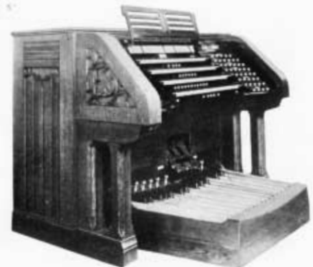
CONGREGATIONAL CHURCH WEST NEWTON, MASS. 45 Stops 7½ H. P. multi-pressure "Orgoblo." Wind pressures, 4 to 10 inches.
