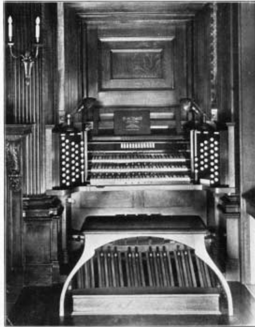
MRS. LUELLA E. STEARNS WYOMING, O. 45 STOPS 7½ H. P. "Orgoblo." Wind pressure, 5 inches.
