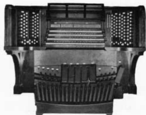
BRICK PRESBYTERIAN CHURCH NEW YORK CITY 97 Stops 30 H. P. multi-pressure "Orgoblo." Wind pressures, 7½ to 20 inches.
